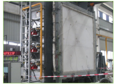
Fire testing to Soben® MP-1000/MultiPro® partition
