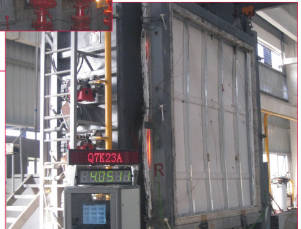
FP®-900/FirePro® under fire tests of ceiling and partition to international standards
